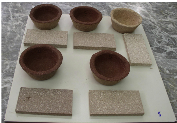
Fig. 3. Crucibles and samples refractories elaborated from Moroccan geomaterials. Sintering temperature 1600 °C.
