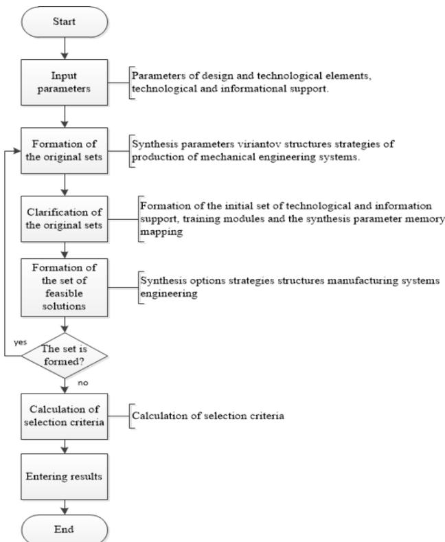
Fig. 2. The general algorithm of the automated decision support system.
