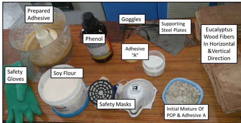
Fig. 1. Ingredients and supporting material used to manufacture the plyboard (Note: PoP is Plaster of Paris)
