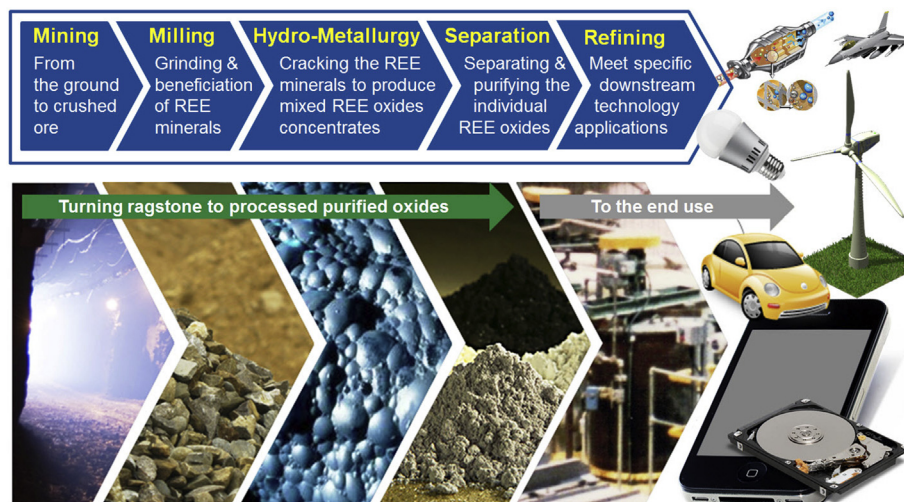
Fig. 4 – The rare earth element complete supply chain.
