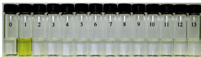
Fig. 10. Colour change of polymer 11 upon the addition of various metal ions in pure water. The numbered vials are labeled as follows, 0: blank, 1: \text{Ag}^+ , 2: \text{Hg}^{2+} , 3: \text{Pb}^{2+} , 4: \text{Mg}^{2+} , 5: \text{Cs}^+ , 6: \text{Li}^+ , 7: \text{Cd}^{2+} , 8: \text{Ca}^{2+} , 9: \text{Fe}^{3+} , 10: \text{Ni}^{2+} , 11: \text{Cu}^{2+} , 12: \text{Zn}^{2+} , and 13: \text{Co}^{2+} . The concentrations of polymer 9 and the metal ions are 5 \times 10^{-6} M and 1 \times 10^{-5} M, respectively [42]. Reprinted with permission from Macromolecules, 44, Qin C, Wong W-Y, Wang L, "A water-soluble organometallic conjugated polyelectrolyte for the direct colorimetric detection of silver ion in aqueous media with high selectivity and sensitivity", 483–489. Copyright (2011) American Chemical Society.
