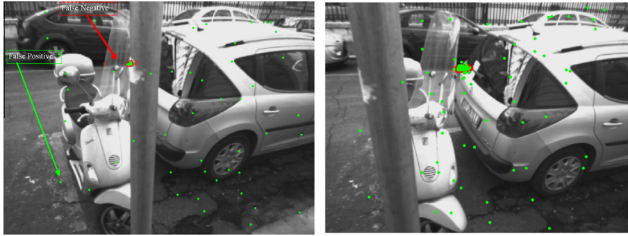
Fig. 15 Results of features and classification validation for the outdoor experiment looking for car fines . In red the PORs, and the coherent patches, in green the estimated point saliency, for the specific task.
