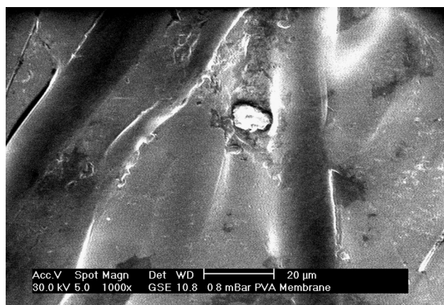
Figure 3 SEM image of PVA membrane.
