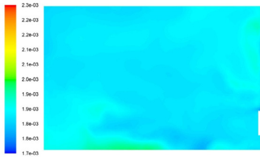
Fig. 6. Simulated CO 2 concentration after 8 hour long sleep. One person in room, V=20.7 m 3 , ventilation flow rate 2 l/s. Vertical A-A (Fig. 2) cross-section
