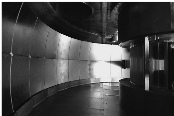
Fig. 12. Si(111) analyzer banks (from left side to center) and the position sensitive ^3\text{He} gas detector (PSD)-amplifier units (right side) in DNA vacuum vessel. Sample position is at the center of PSD-amplifier units.
