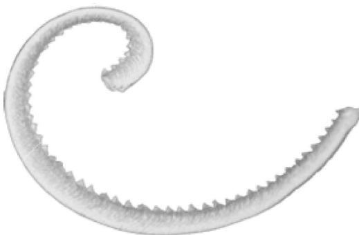
Fig. 2. Example of the chip shape for the cutting speed v_c = 200 m/min
