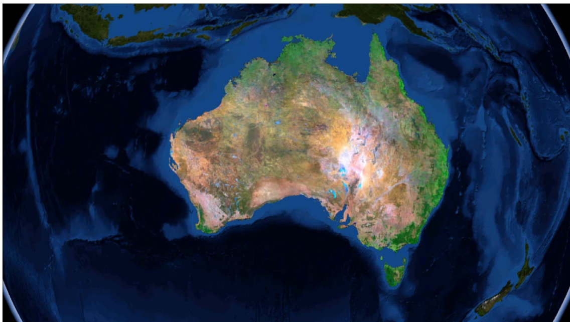
Fig. 1. Animation of the 25 m Australian Reflectance Grid (ARG25) across the Australian continent showing seasonal variations throughout the year. Continental mosaics were produced using temporal stacks of ARG25 data from 2000 to 2011.
