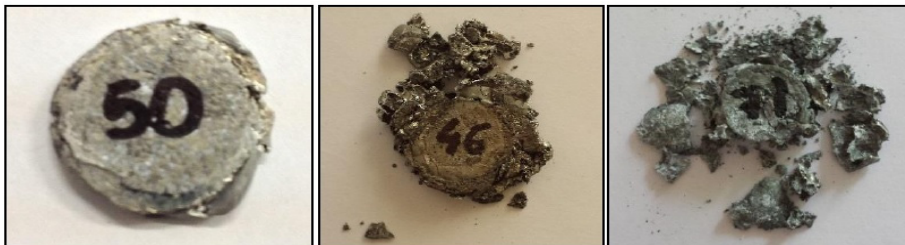
Fig. 4. pure Al (a), in AlSi6 (b) and in AlSi8 (c) foams after deformation.
