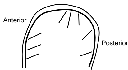
Fig. 8. Reproduced from Ref. 16 shows the dominant c-axis polar orientation inferred by comparing \Delta n values for different illumination directions that are confined to the sagittal plane (retardance images not shown).
