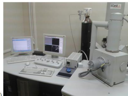
Fig. 2. Microscopes used in the experimental study: (a) Nikon SMZ 800 and (b) Quanta 200
