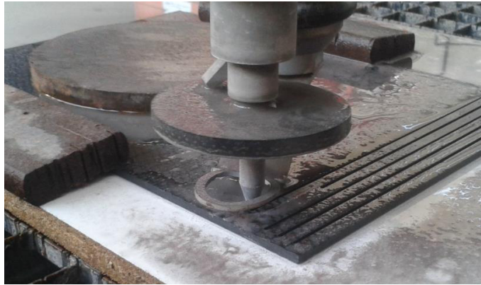
Fig. 1. Detail cutting machine using water jet machining a CFRP plate
