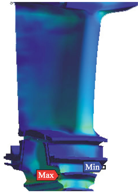
Figure 12 Stress analysis results for 1st stage blade.
