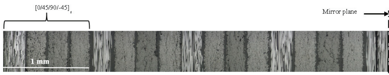
Figure 1. Microstructure of M21/T700 composite laminate
