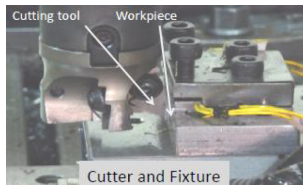
Fig. 1 Experimental set-up for interrupted orthogonal cutting (milling)
