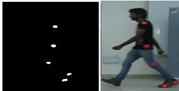
Fig.6. Marker detection scheme and its corresponding position in System
