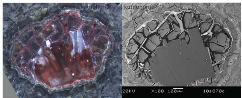
Figure 6. Optical microphotograph (left) and SEM microphotograph (right) of post reacted basalt removed from the top of CRB-6 (31 MPa and 137^\circ\text{C} ) showing the carbonate precipitate forming inside pre-existing small vesicles containing secondary minerals (chlorite, cristobalite, and heulandite).
