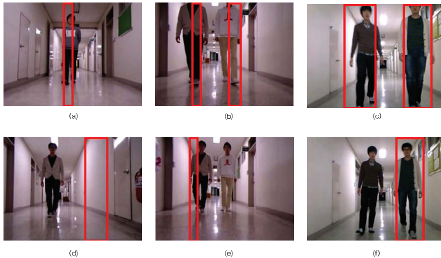
Fig. 4. Experimental results: Successful cases are shown in (a), (b) and (c), while detection failures are presented in (d), (e) and (f).
