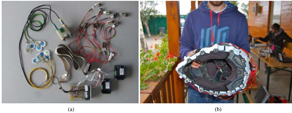
Fig. 1. (a) overview of the sensor and data logging device setup for both sEMG and contact measurement; (b) sensors attached to the underside of a motocross helmet.
