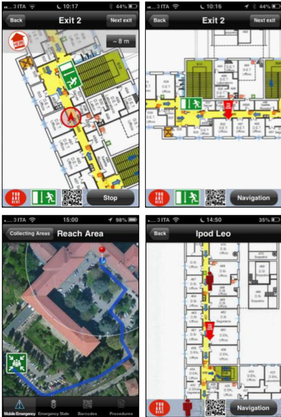
Fig. 7. In the order: indoor navigation to reach an exit, outdoor navigation segment, indoor navigation to reach a colleague.
