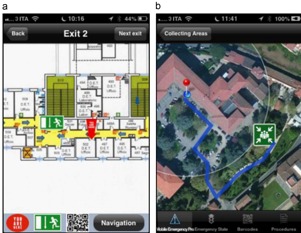
Fig. 4. (a) The indoor path manager displays the path suggested to reach an emergency exit. (b) The outdoor path manager shows the suggested path to reach an outdoor collecting area.
