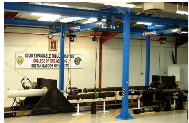
Fig. 7. Expandable Test Rig (ETR) at Engineering Research Lab (ERL), SQU.
