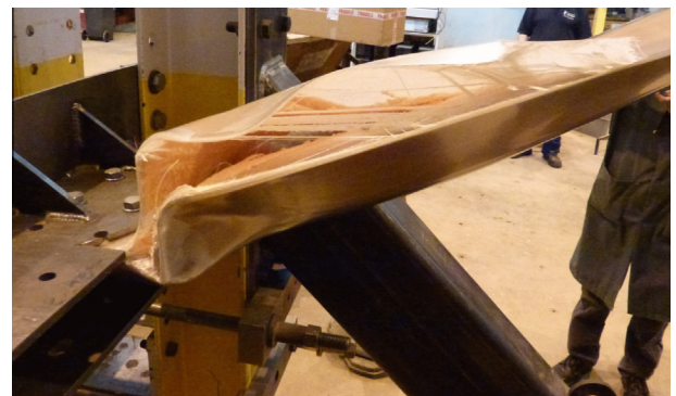
Fig. 11. The E-glass blade, failing at the blade root, exhibited extensive delamination.
