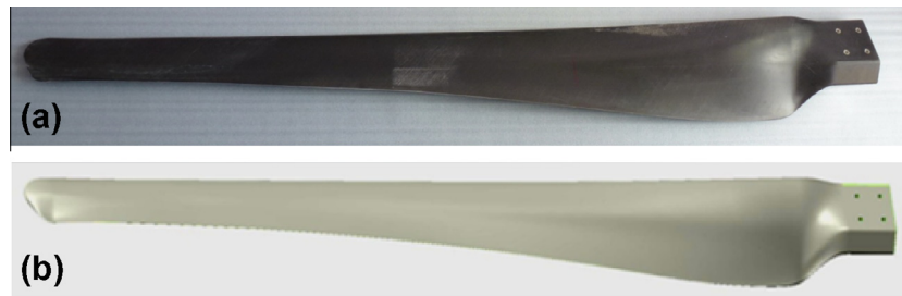
Fig. 3. Images of the (a) flax/polyester and (b) E-glass/polyester blades.
