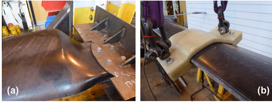
Fig. 5. Image showing the (a) test rig and (b) composite saddle.
