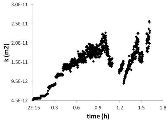
Fig. 4. Variation of fracture permeability with time in a sandstone core. The flow rate was 60 mL h<sup>-1</sup>.
