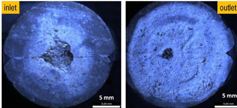
Fig. 3. Frontal views of inlet and outlet of a limestone core. Brine circulated through the fractured core at 5 mL h<sup>-1</sup>.
