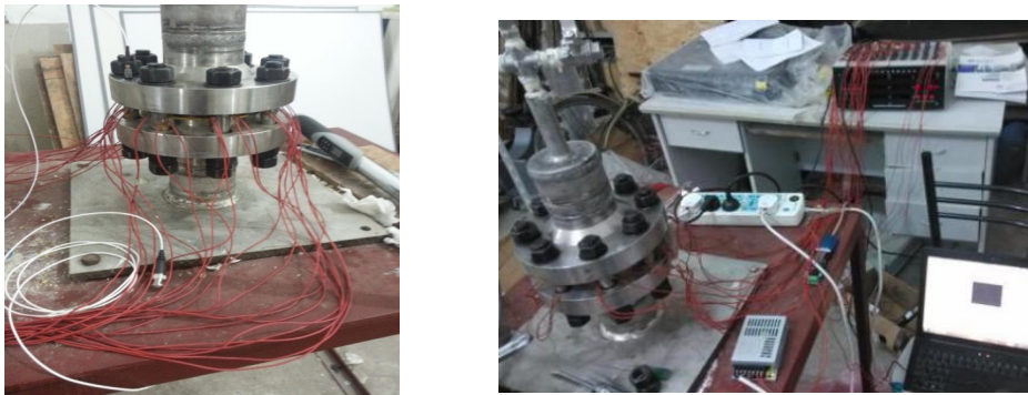
Fig.11. Measurement device for Bolt loads and flange leak rate.
