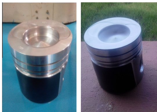
Figure 2 Snapshots of uncoated baseline engine piston (left) and YSZ coated piston (right).
