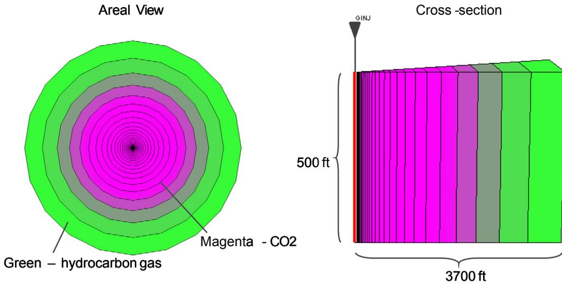
**Figure 3 Simulation model showing CO2 distribution after one year**
