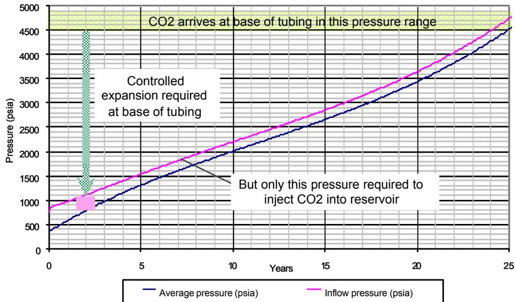
**Figure 6 Pressure at base of tubing compared to reservoir pressure response**
