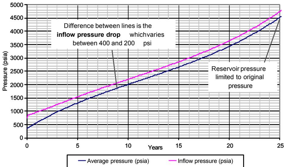
**Figure 4 Reservoir pressure response to CO2 injection**
