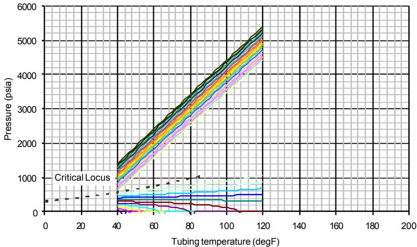
**Figure 7 Tubing pressures assuming injection temperature of 40°F (4.4°C)**
