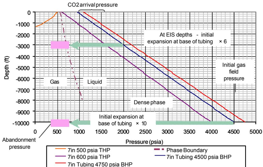
**Figure 5 Pressure in injection well tubing during CO<sub>2</sub> injection**
