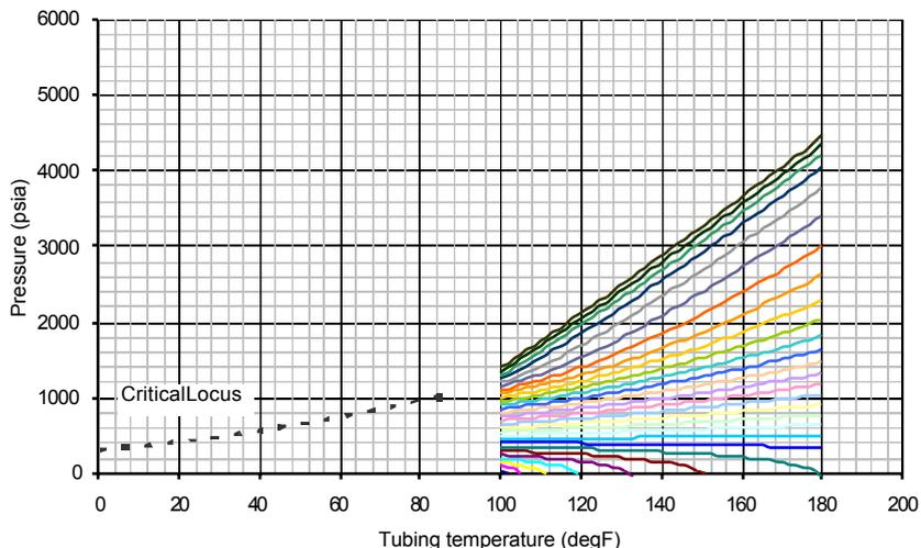
**Figure 8 Tubing pressures assuming injection temperature of 100°F (38°C)**
