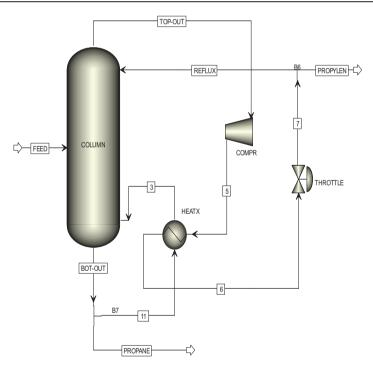
Figure 1. Flowchart of tower liquid flash reboiling heat pump distillation system by Aspen Plus
