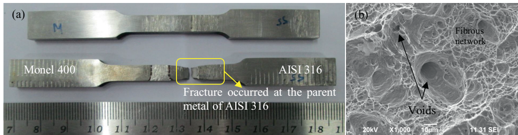
Fig. 4 (a) ASTM E8 standard tensile samples and the fracture sample (b) SEM fractograph of the fractured sample
