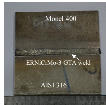
Fig. 1 Macro-photograph of the GTA weldments of Monel 400 and AISI 316
