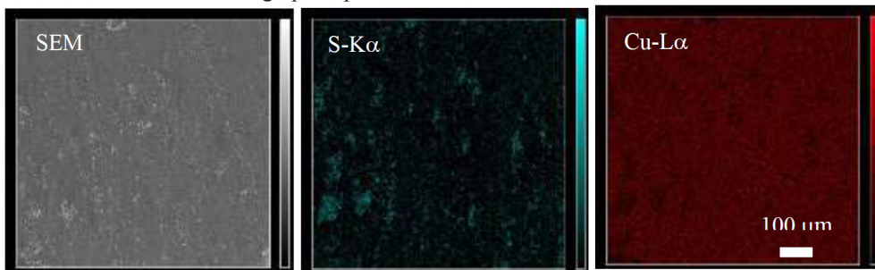
Fig. 1. SEM/EDX images of sulfide containing Cu alloy
