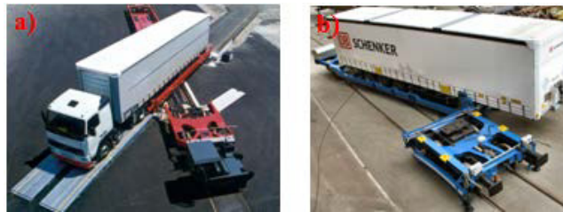
Fig. 1. Wagons for trucks semitrailers transportation: (a) developed by French company Moda Lohr and (b) Megaswing developed by Swedish company Kockums Industrier, www.[...] (2009). www.[...] (2011).
