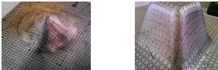
Fig. 7 Formed truncated square pyramid and cone with grid pattern
