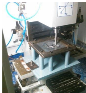
Fig. 3 Fixture with sheet metal mounted on CNC machine
