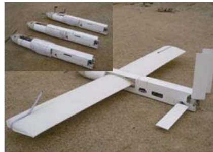
Fig. 4 Inflatable wing in packed and deployed configuration.
