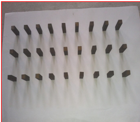
Fig.3. Pieces lying in vertical after WEDM
