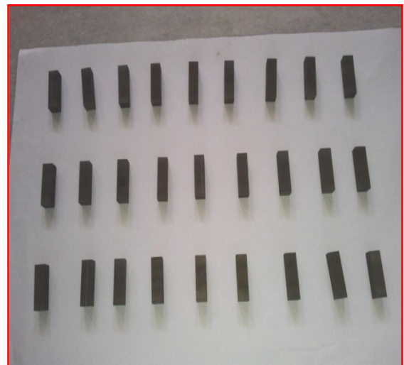
Fig.4. Pieces lying in horizontal after WEDM
