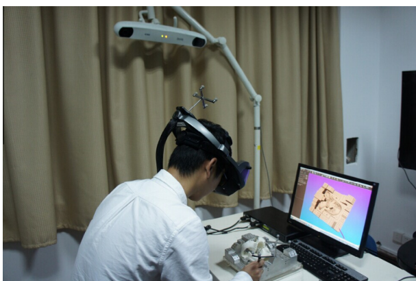
Fig. 8. The accuracy verification of AR-based surgical navigation system.
