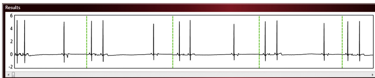
Fig. 7. Graphical results as displayed in the Data Insights Results Wave View from a heart rate change search executed on an ECG signal from a canine. In this example, instances of sinus pause were located.
