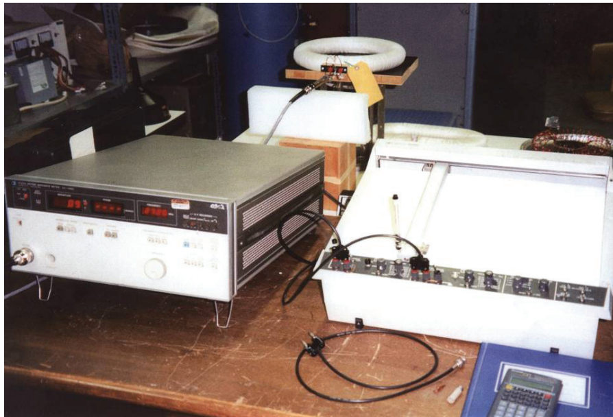
Figure 4. Typical equipment (HP impedance analyzer and plotter) for detecting resonant toroid frequencies.
