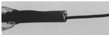
Figure 1. Angioscope (Advanced Cardiovascular Systems) showing a guide wire (right) through the distal flush lumen, illumination fibers and imaging bundle (left) at the tip of the 1.4 mm diameter catheter.
