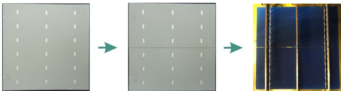
Fig. 1: Full cell before laser scribing (left), full cell after laser scribing and before breaking (middle), and two half cells positioned on the measurement stage (right).
