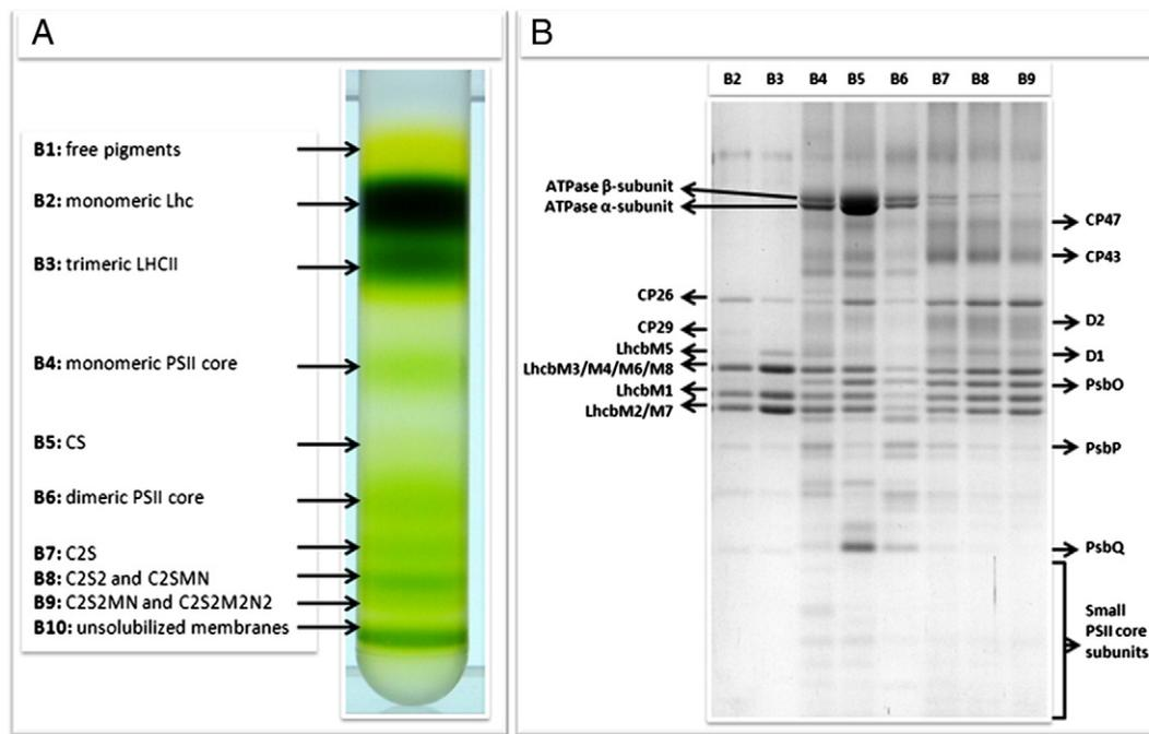
**Fig. 1.** Purification of PSII sub- and supercomplexes. Panel A: fractionation of PSII sub/super-complexes by sucrose density gradient. Panel B: SDS-PAGE analysis of fractions B2–B9 from sucrose gradient. Proteins identified by mass spectrometry are indicated.
