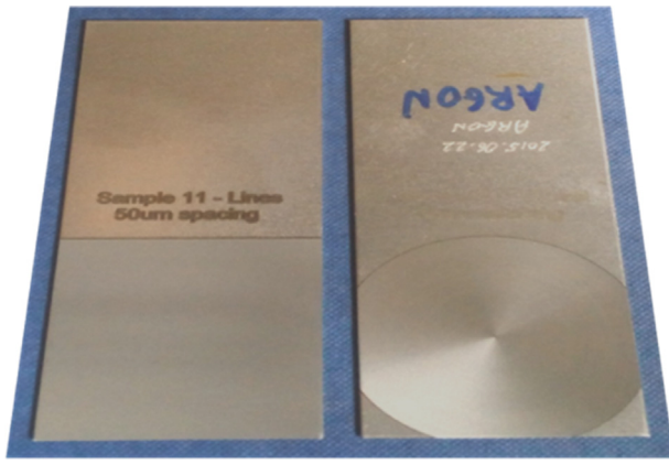
Fig. 2. Steel coupons with the laser-generated textures containing 30 µm deep parallel troughs (left) and a 30 µm deep spiral trough (right).
