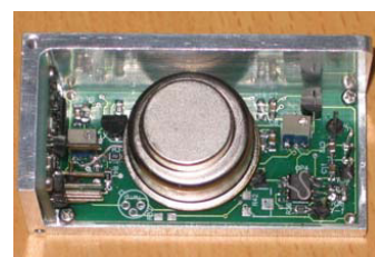
Fig. 6: Photograph of the packaged resonant pressure sensor with a circuit.
