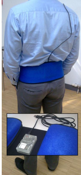
Fig. 1. Posterior view of the placement of the inertial measurement unit (IMU), the unit was placed on the lower back by using a double sided adhesive tape with a band. The figure shows as well the inertial unit fixed on the band
