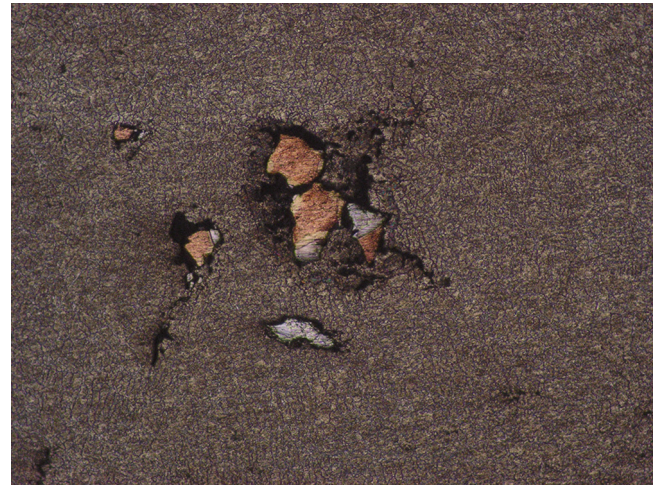
Fig. 5. Clustering of particulates, Al–15% Cu composite, 100 ×.
