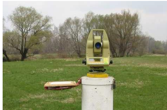
Fig. 5. Total station on the baseline in Hlohovec
