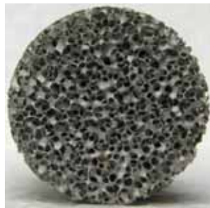
Fig. 2. View of tested FEC foam: a) channel packing; b) pore structure
