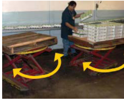
Fig. 7. Turntable on a load leveler [12].
