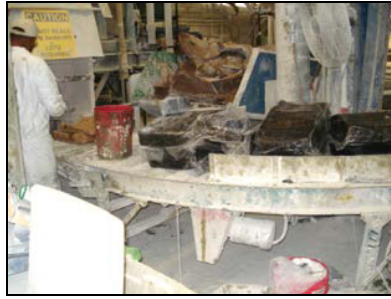
Fig. 4. Placing rubber batches on conveyor belt.
