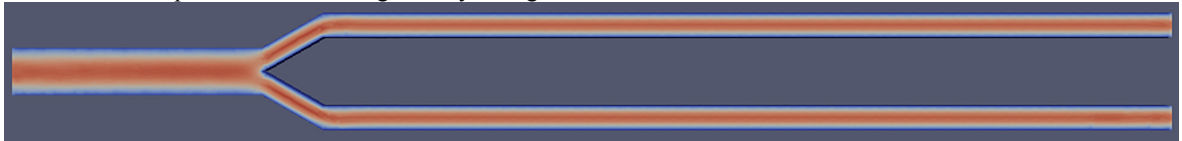
Fig. 3. Y shaped geometry. The inlet of the fluid is in the left of the geometry and there are two outlet branches in the right side. The angle between the two outlet branches is 60° degrees. The diameter of the main and outlet branches are 2.5mm and 1.125mm, respectively. The overall length of the simulated geometry was 0.06 m and the computational grid was composed by 5644 prism cells.
