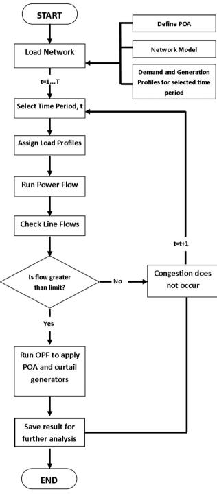
Fig. 2. Constraint analysis modelling process.
